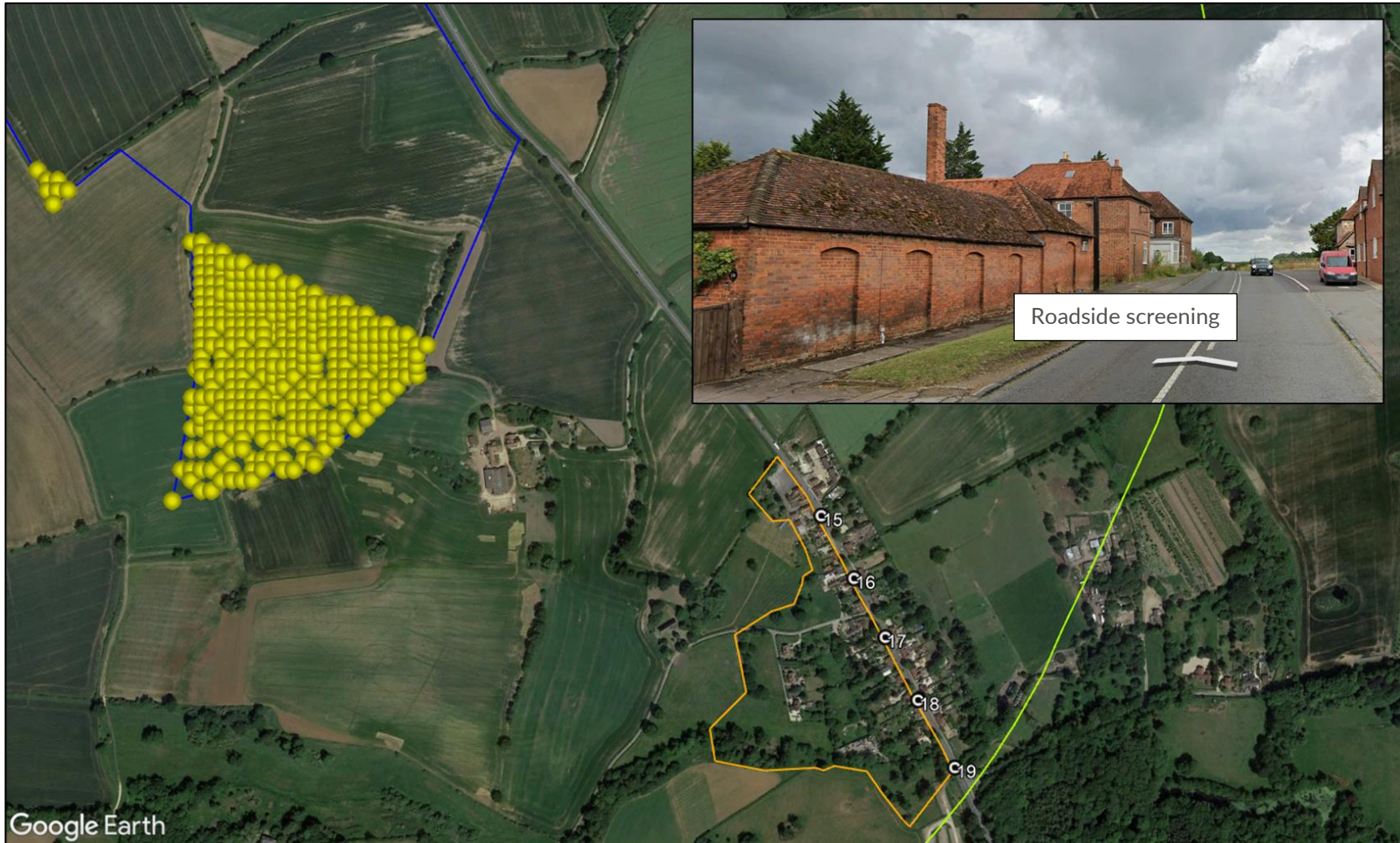
Figure 12 Screening for road receptors 15-19 with street view inserts from receptor 15
